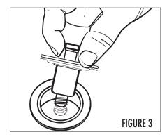
Pull out stopper, clean hair from drain and re-install stopper
